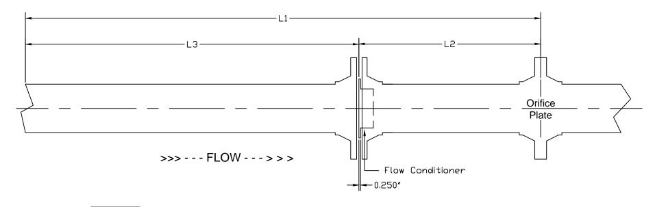
Description Range Rec  $17D_n$  $L1 \ge 13D_n$ Distance from meter run valve or piping disturbance to orifice plate 7D<sub>n</sub> Distance from flow conditioner to L2 5-11D<sub>n</sub> orifice plate ≥5D<sub>n</sub> Distance from meter run valve or  $L3 \ge 5D_n$ piping disturbance to flow conditioner pin location
